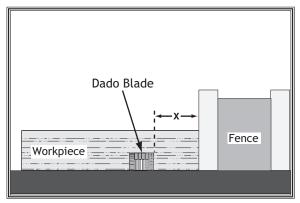
Figure 49. Illustration of a dado cut.
